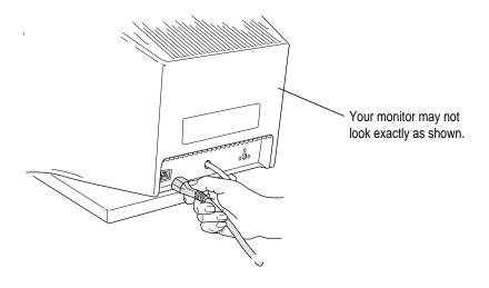
Plug the other end of the power cord into the monitor power socket on the back of your computer.
